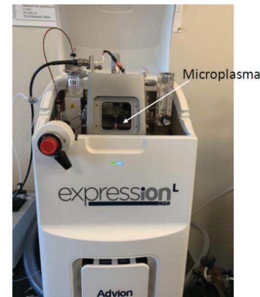
Liquid sampling-atmospheric pressure glow discharge (LS-APGD) microplasma integrated with an Advion Compact Mass Spectrometer (CMS) for at-reactor elemental analysis.
